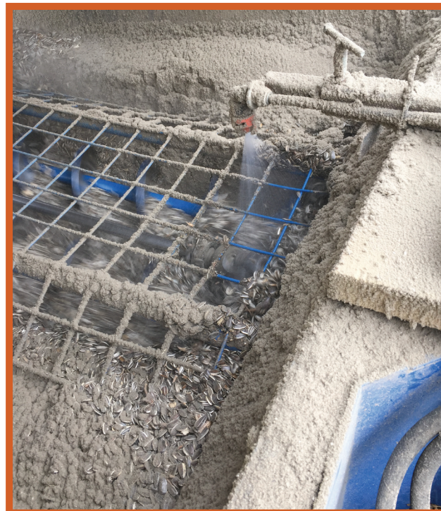
Edinger applies Diacon® IGR directly to the grain stream as the commodity is loaded into storage.
